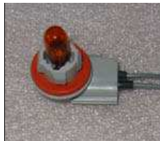
Wires soldered onto bulb holder
