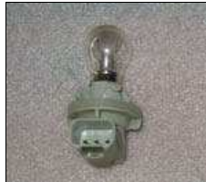
Top Bulb - UK Stop/rear light 3 pins, Ground, Major & Minor
