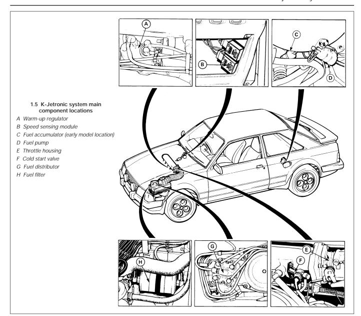
The fuel accumulator has two functions, (i) to dampen the pulsation of the fuel flow, generated by the pump and (ii) to maintain fuel pressure after the engine has been switched off. This prevents a vapour lock developing with consequent hot starting problems.
